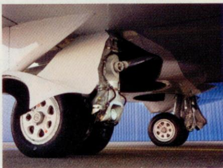
Bombardier's Challenger 605 on the ramp at Hartford service center (top). The wing and tail both begin flying at the same time during the takeoff run, so liftoffs are smooth. The 605's anti-skid brakes have been beefed up with an additional rotor (above). The landing gear is hydraulically actuated, but free-falls for emergency extension. But that's not likely—the 605's hydraulic system has six hydraulic pumps for redundancy.
